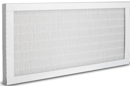
F7 is classified as a fine filter according to EN 779:2012 norm and as ePM<sub>1</sub> 55% in accordance with new standard ISO 16890.
