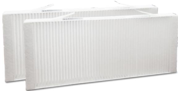
G4 pleated panel filters create a larger media surface area for air filtration and ensure lower pressure drops. Filters are classified as in the ISO Coarse 70% according to ISO 16890 standards.
