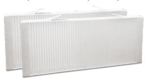
G4 pleated panel filters creates a larger media surface area for air filtration and ensures lower pressure drops. Filters are classified as in the ISO Coarse 70% according to ISO 16890 standards.
